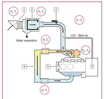
Figure 4. Generic Air Intake System layout
