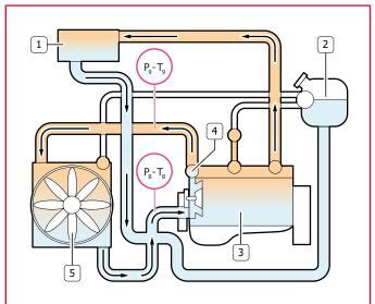
Figure 6. Cooling system with expansion tank (blue outline indicates rubber hoses)
